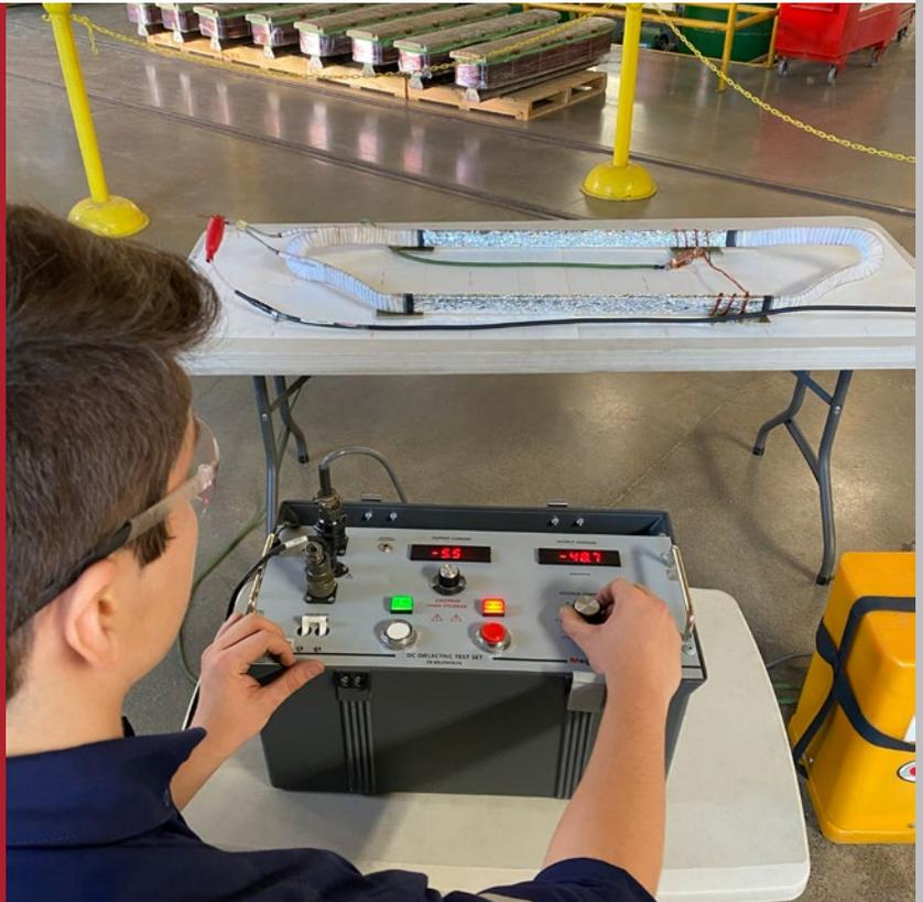
Abstract - Overvoltage tests, also known as high potential or “Hi-Pot”, are used frequently to ensure the minimum dielectric strength of the insulation system. It is not a destructive test, nor does it degrade materials. These tests are carried out in whole or in part of the winding, to test the ground condition of the insulation of rotating electric machines.
