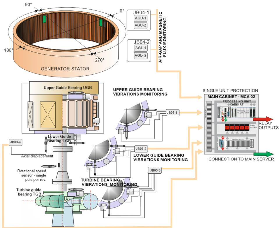
Fig 2. Sensor layout of installed online monitoring system
