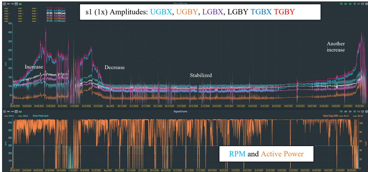
Fig 1 Long-term trends. TOP DIAGRAM: 1x harmonic (relative vibrations peak) for all bearings; BOTTOM DIAGRAM: Rotational speed and active power during the 6-month period.
