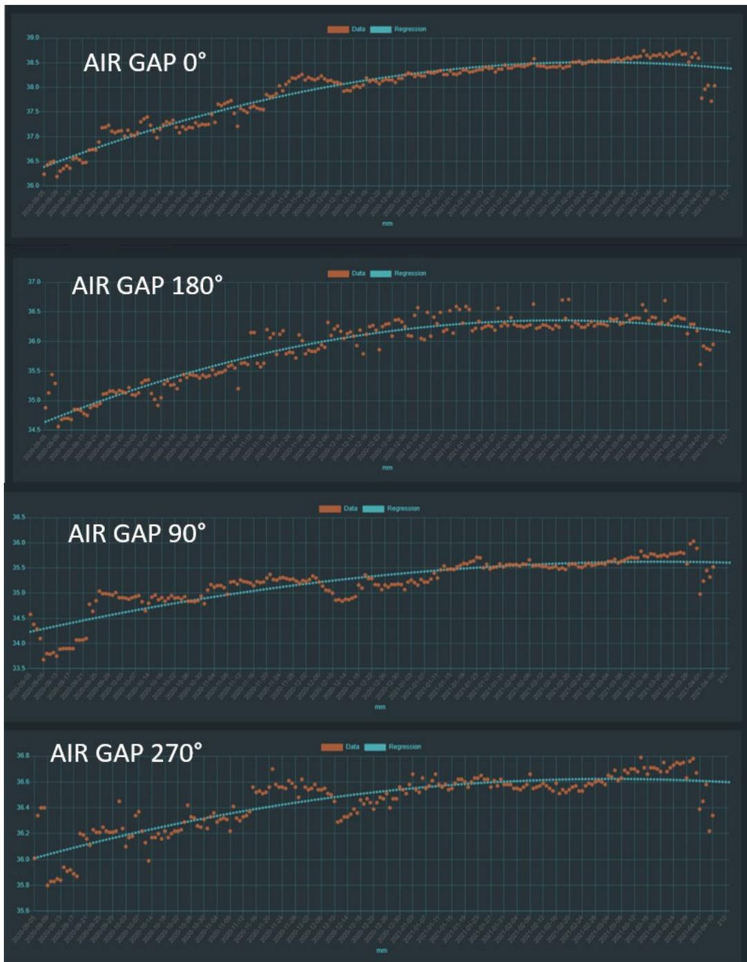
Fig. 5 Average daily (DC) value of an air gap signal, from each sensor, for a 6-month period, filtered to operation at full load.
