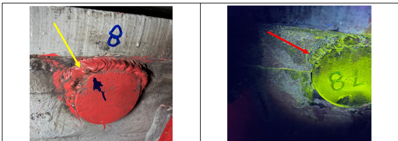
Fig. 13 Linear indication (crack) on securing weld on stator soleplate radial pins.
