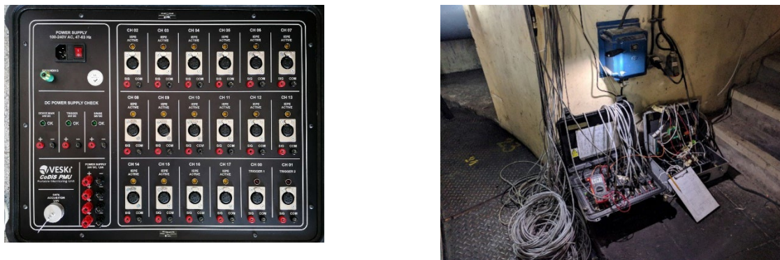
Fig 2. LEFT: Portable Measurement Unit (PMU) – an 18 channel signal conditioning and acquisition device. RIGHT: Two PMU’s running synchronously with all signals connected. Photo from the power plant.
